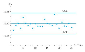
**Figure 16.2**  $\overline{X}$  chart for the viscosity data of Example 16.1
