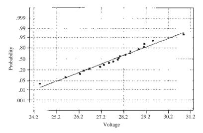
Figure 4.36 Normal probability plot of the breakdown voltage data from Minitab
