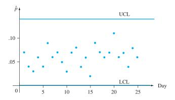
Figure 16.5 Control chart for fraction-defective data of Example 16.6
