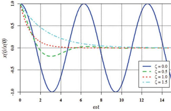
**Figure 6.** Behavior of damped harmonic oscillator with different damping modes.
