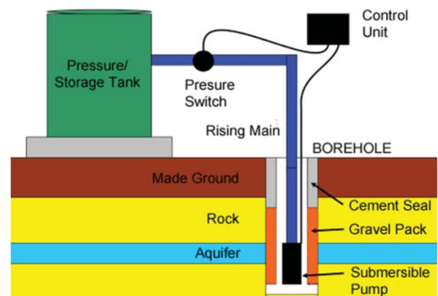
**Figure 2.** Illustration of borehole and water flow. Picture from <http://www.waterseekers.co.uk/borehole-drilling-faq.php#&panel1-1>.
