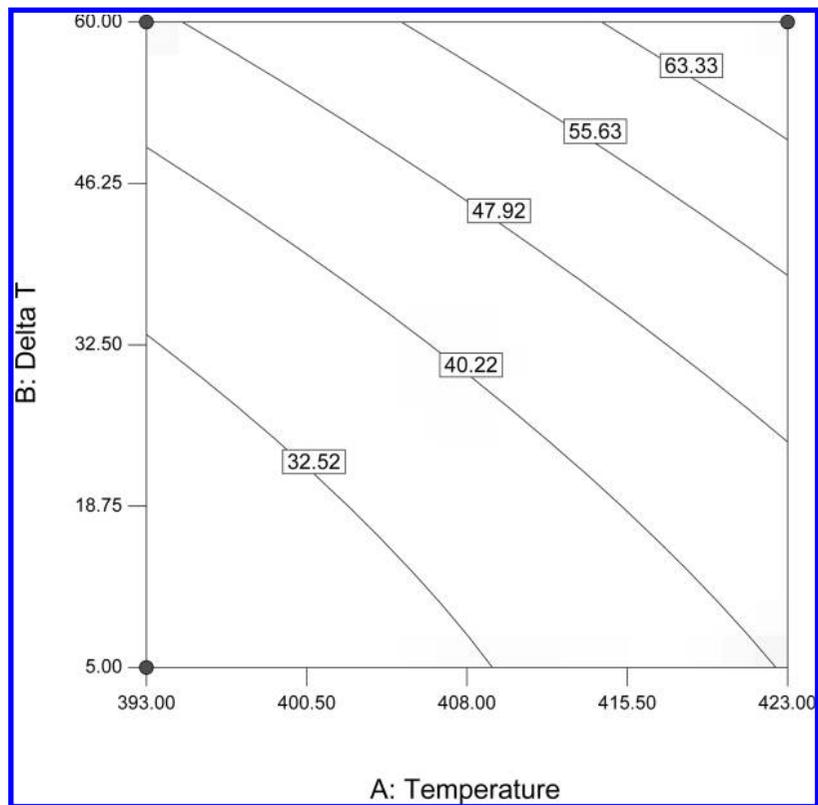
Figure 6. DEG:TEG selectivity ratio as a function of  $T$  and  $\Delta T$  for EG:EO = 6 and CC = 0.06.
