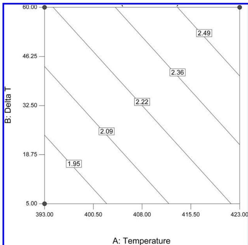
Figure 5. SD (DEG:TEG) as a function of  $T$  and  $\Delta T$  for EG:EO = 6 and CC = 0.06.
