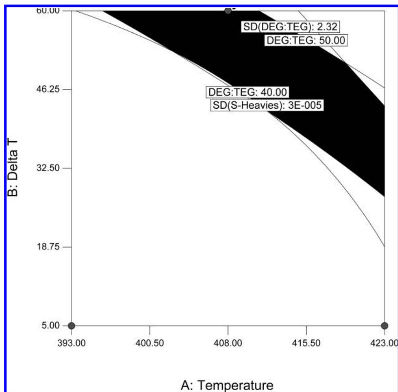
**Figure 8.** Contour overlay plot of the transmitted SD and selectivity of the calculated products, that is, DEG:TEG ratio and S-Heavies (feasible area in black).
