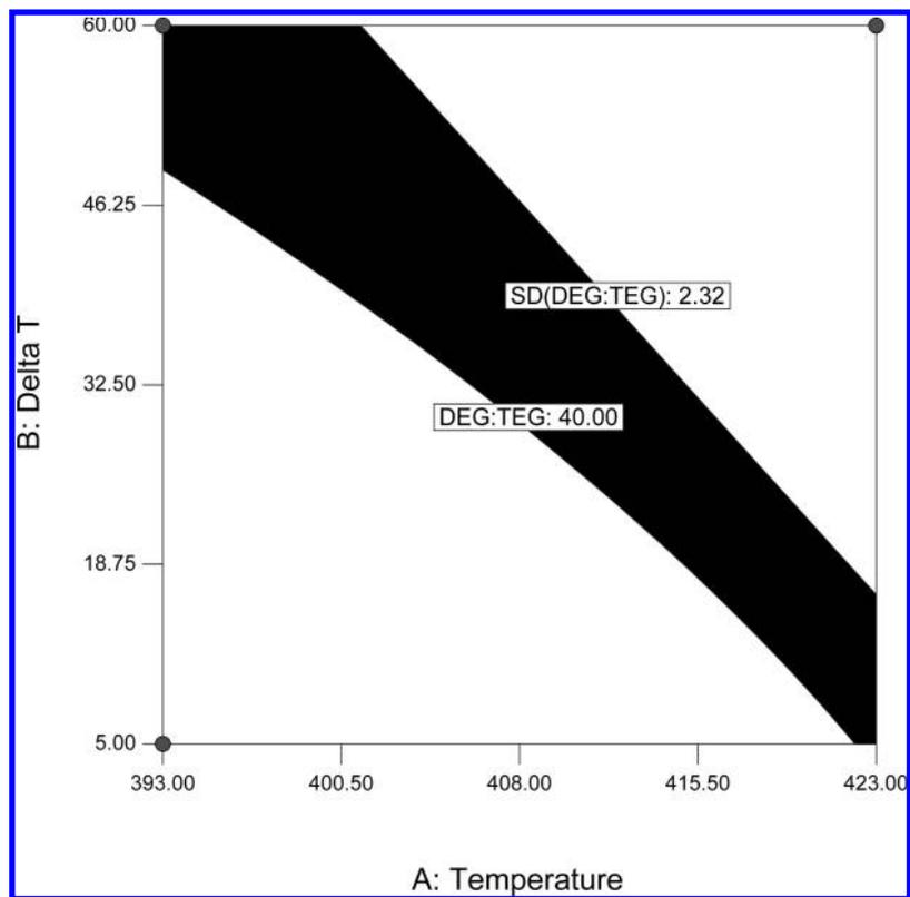
Figure 7. The feasible operating area for criterion (22) for  $c = 2.32$ , but with a DEG:TEG ratio greater than 40 (feasible area in black).
