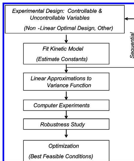
**Figure 1.** Schematic diagram of robustness studies utilizing the kinetic or fundamental model.
