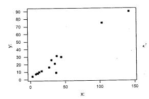
There is a strong linear relationship between BOD mass loading and BOD mass removal. As the loading increases, so does the removal. The two outliers seen on each of the boxplots are seen to be correlated here. There is one observation that appears not to match the liner pattern. This value is (37, 9). One might have expected a larger value for BOD mass removal.
